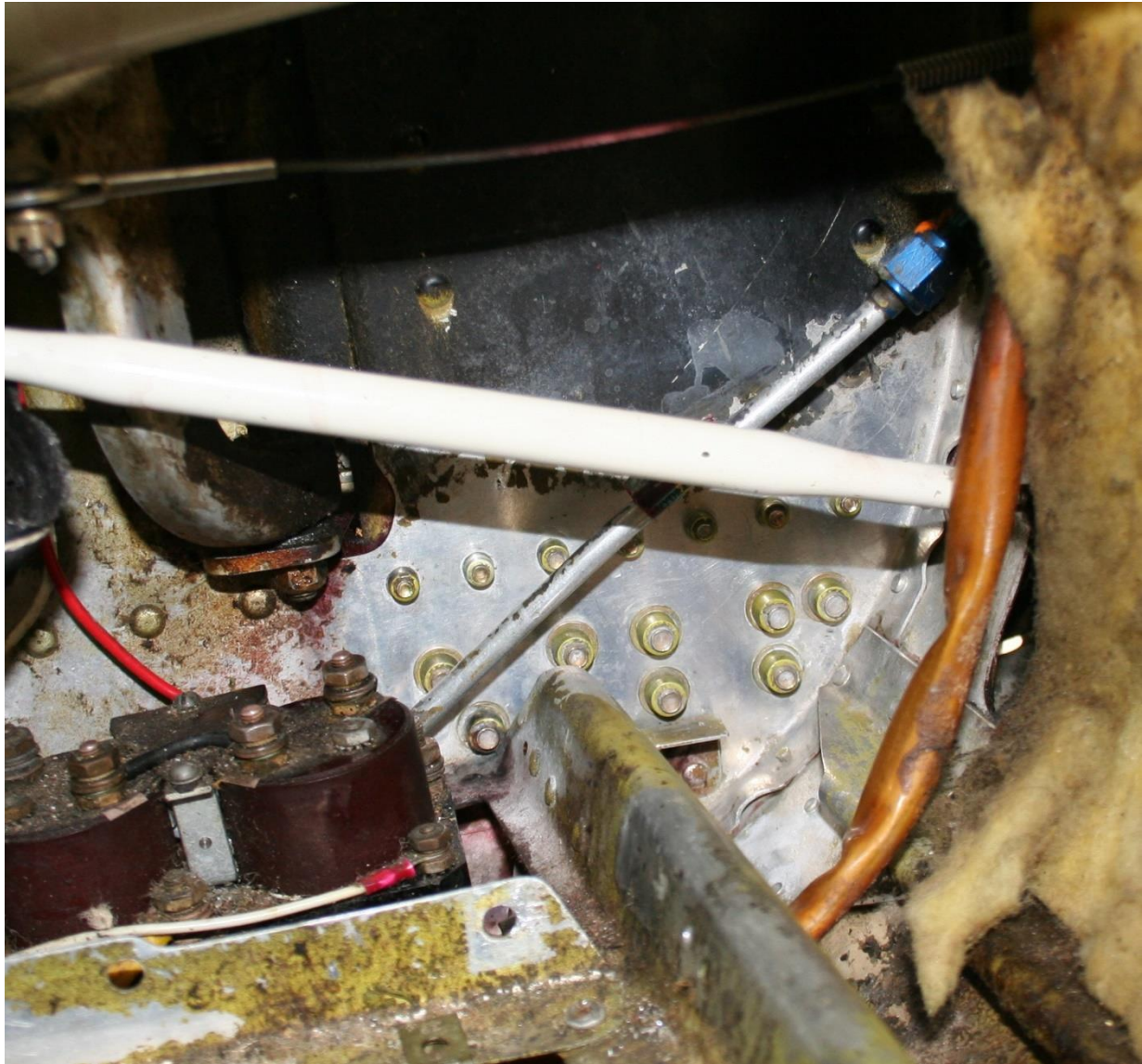
Rear View Of Right Side Spar
